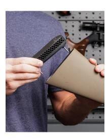
**Step 1.**Remove the butt pad screws with a #2 Phillips screwdriver and pull the butt pad from the stock.
