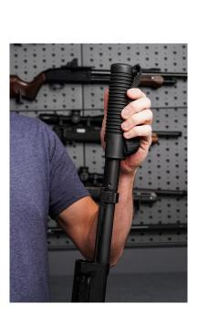
**Step 4.**Slide the pump off the action tube.
