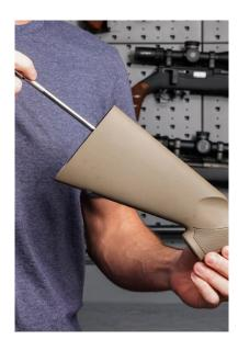
**Step 2.**Remove the bolt that secures the stock to the action with a 1/2" socket and long extension. Remove the stock.
