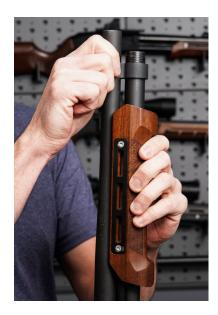
**Step 7.**Slide the barrel over the action tube. Move the fore end rearward so the barrel seats completely.
