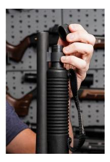
**Step 1.**Remove the action tube cap by unscrewing counter-clockwise.
