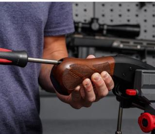
**Step 3.**Align the Club Grip with the hole in the rear of the receiver. Insert the hex screw and tighten until secure.
