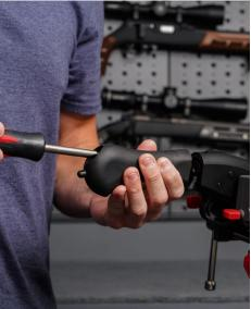
**Step 2.**Remove the screw that secures the stock to the action. Remove the stock.
