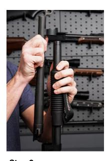
**Step 2.**Sliding the fore end rearward to relieve tension on the barrel.
