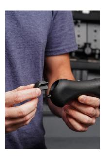
**Step 1.**Using a flathead screwdriver, pry open the cover on the rear of the Shockwave and remove.
