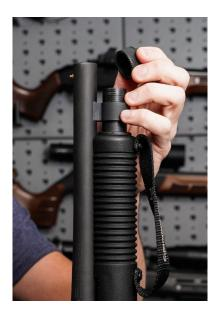
**Step 1.**Remove the action tube cap by unscrewing counter-clockwise.
